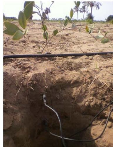
Moisture and salinity probes inserted into the root zone of Jojoba
