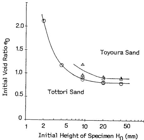
Fig.4: Relationship between the initial void ratio and the initial height of specimen.
