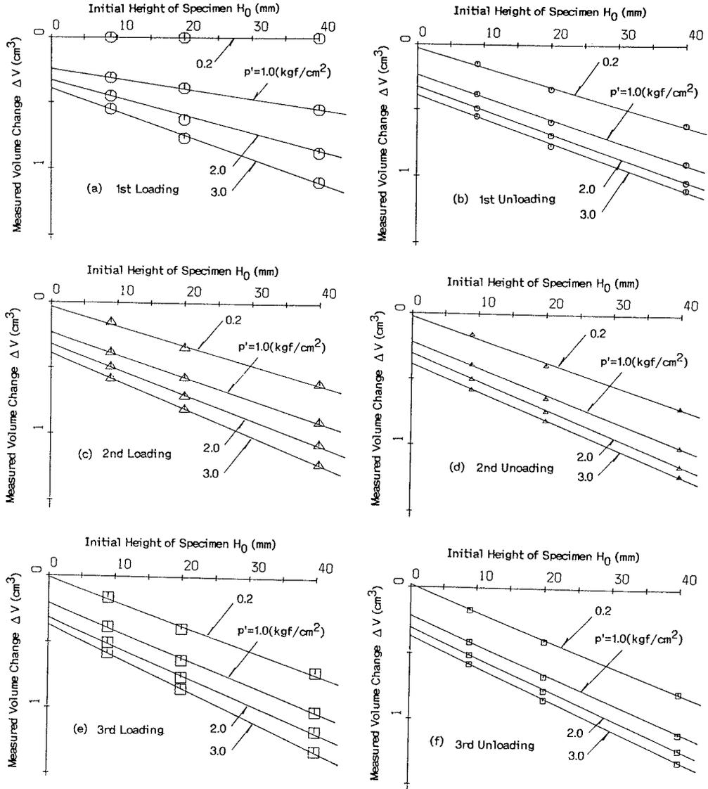
Fig.6: The relationship between the measured volume change and the initial height of specimen for each loading/unloading stage.
