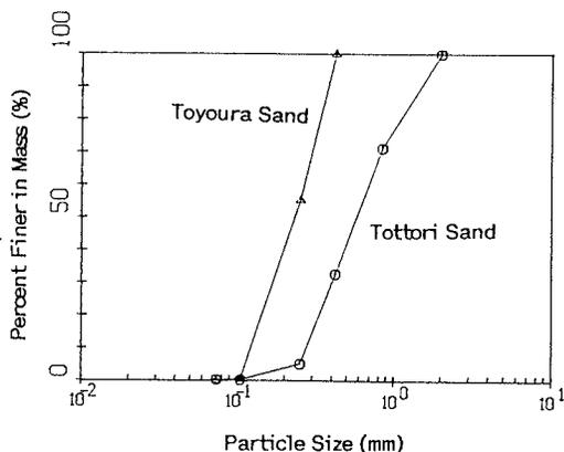
Fig.3: The particle size distributions for the samples used.
