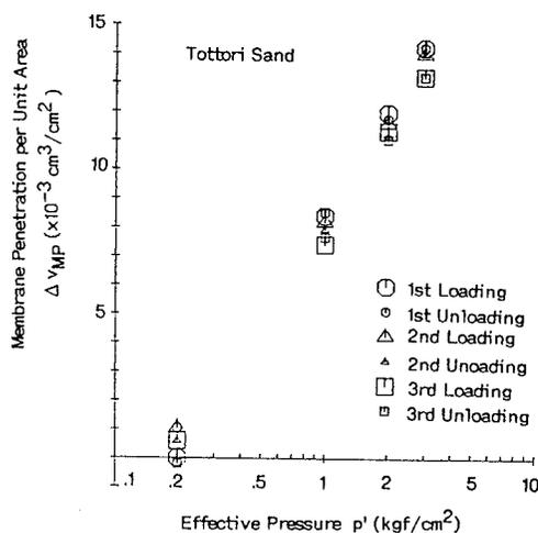
Fig. 7: The membrane penetration per unit area of membrane vs. the effective pressure.
