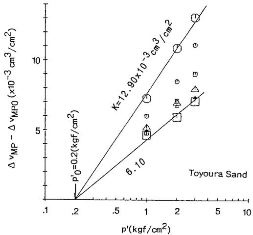
Fig.11: The relationship between the change in the membrane penetration,  $\Delta v_{MP} - \Delta v_{MP0}$ , and the effective pressure.
