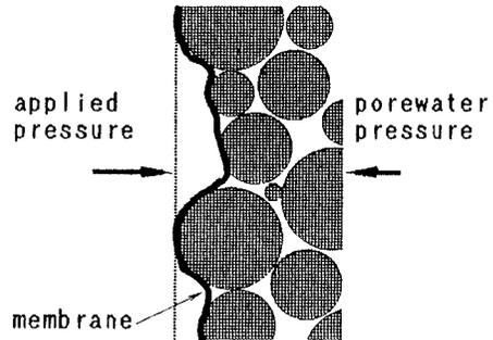
Fig.1: Schematic representation of the membrane penetration.
