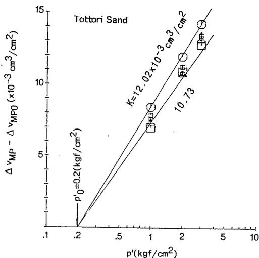
Fig. 8: The relationship between the change in the membrane penetration,  $\Delta v_{MP} - \Delta v_{MP0}$ , and the effective pressure.
