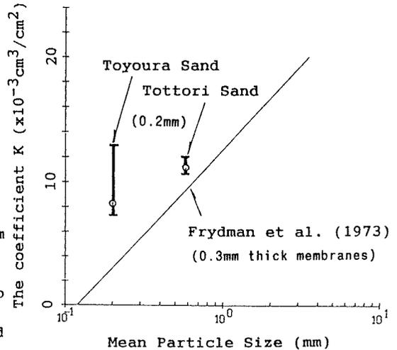
Fig.12: The relationship between the coefficient K in Eq.(3) and the mean particle diameter of the samples.
