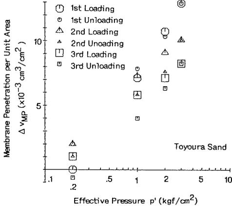
Fig.10: The membrane penetration per unit area of membrane vs. the effective pressure.(Toyoura Sand)
