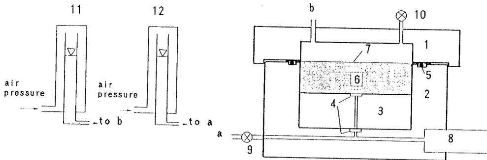
1 upper mold; 2 lower mold; 3 spacer disc; 4 porous stones; 5 O-ring; 6 specimen; 7 membrane; 8 porewater pressure transducer; 9 drainage valve; 10 air-release valve; 11,12 air-/water-pressure transformation instruments (volume change measurement instruments)
