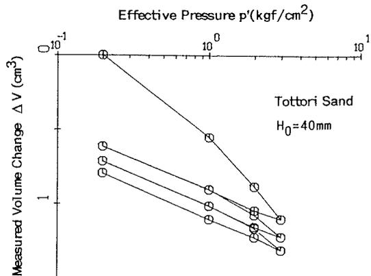
Fig.5: The measured volume change for Tottori Sand.
