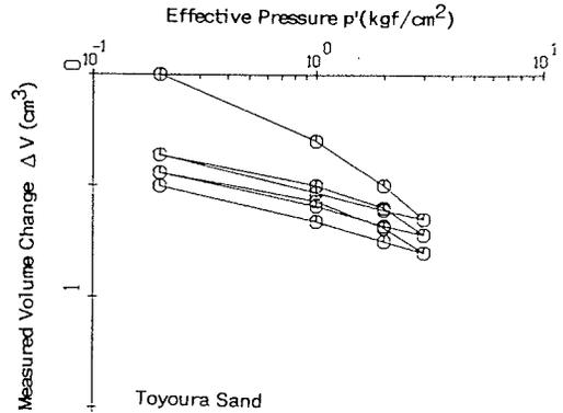
Fig.9: The measured volume change for Toyoura Sand
