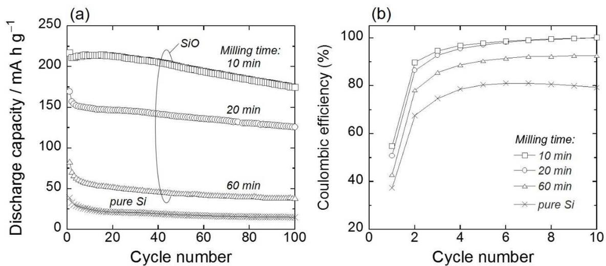
Fig. 4 (a) Cycle performance of electrodes consisted of milled SiO powder at various times. For comparison, the performance of Si electrode was plotted. (b) Variation in coulombic efficiencies in the initial 10th cycle for their electrodes.
