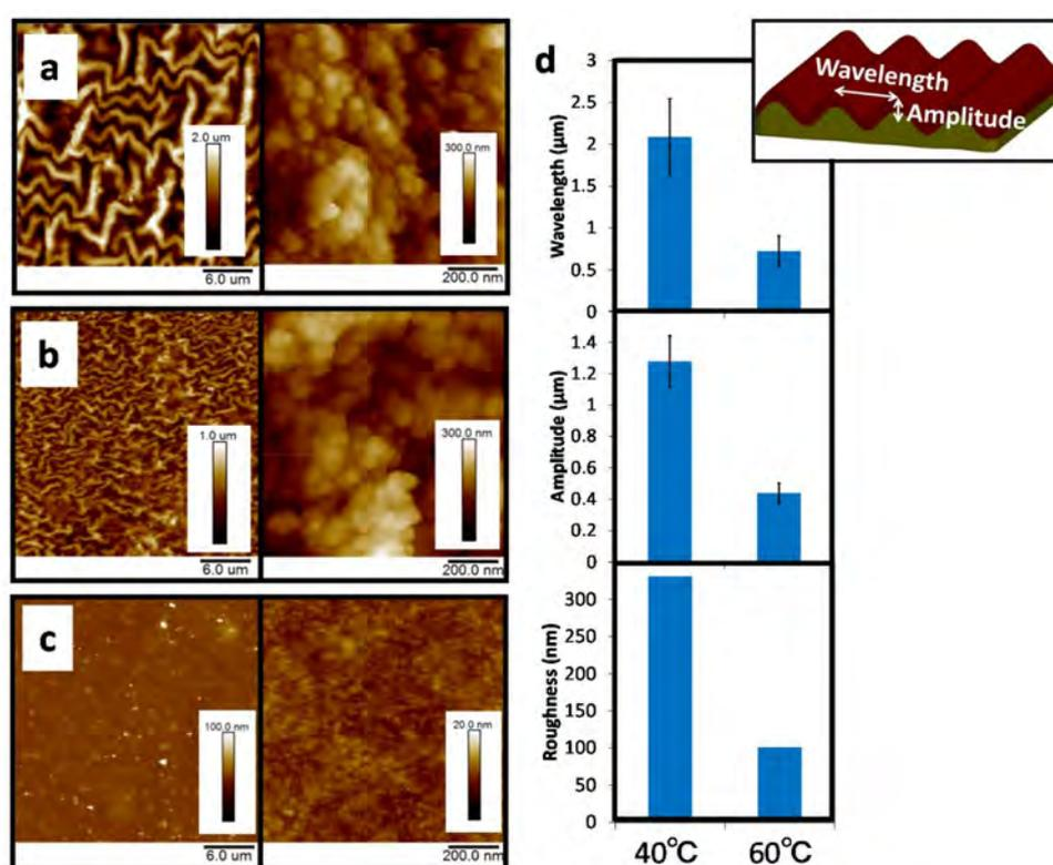
**Figure 2.** AFM images of the wrinkle-CS films prepared via immersion treatment at 40 °C (a) and 60 °C (b); and the original CS film (c) under atmospheric conditions and detailed characterization of the wrinkles (d). Error bars reflect the standard deviations.
