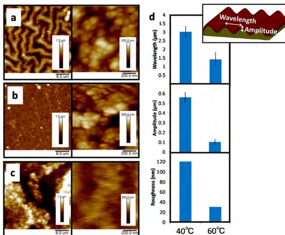
**Figure 3.** AFM images of the wrinkle-CS films prepared via immersion treatment at 40 °C (a) and 60 °C (b); and the original CS film (c) under PBS and detailed characterization of the wrinkles (d). Error bars reflect the standard deviations.
