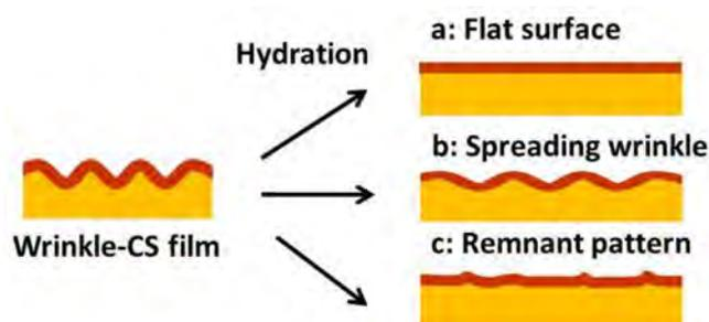
**Figure 4.** Illustration of the hydrated CS film assuming the skin layer completely hydrates (a) and the observed hydration behaviour on the wrinkle-CS films prepared via immersion treatment at 40 °C (b) and 60 °C (c).
