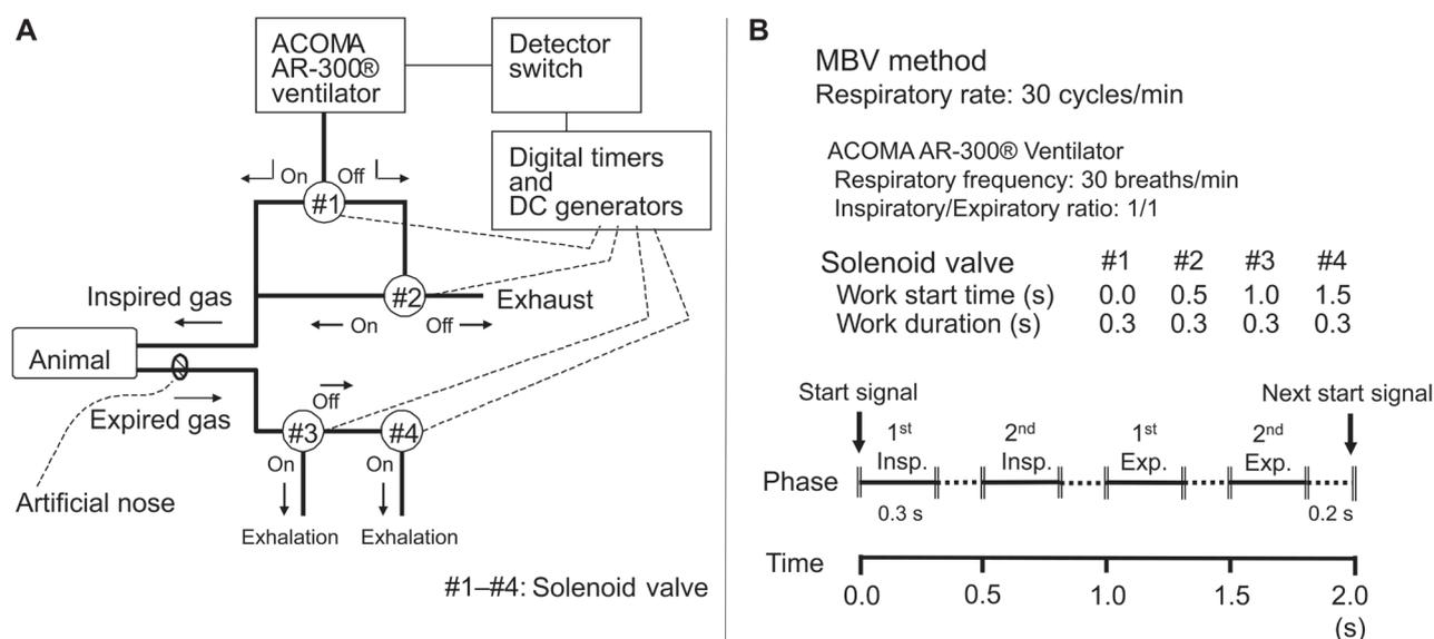
**Fig. 1.** Schematic diagram of the prototype ventilator (A). The setting of the Acoma AR-300 and an example of the time allocation regarding the four solenoid valves, when the respiratory rate is set to 30 cycles/min in the MBV method (B). In the MBV method, the 1st and 2nd inspiratory, and the 1st and 2nd expiratory phases taken together, are defined as one cycle. DC, direct current; Exp, expiratory; Insp, inspiratory; MBV, marathoners' breathing rhythm ventilation.
