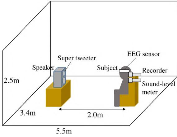
Fig. 1. Measurement environment.
