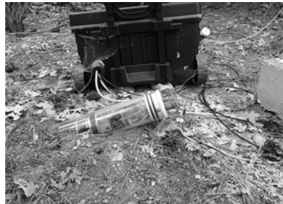
Automated mini-rhizotron set in semi-arid region in James Reserve, California, USA.
