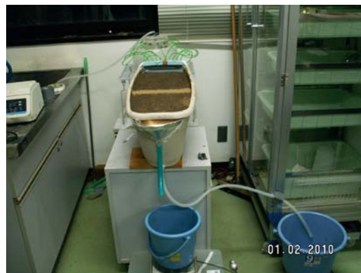
Sand ditch placed in the middle of soil box
