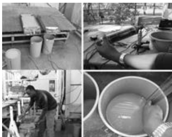
Measurement of runoff, sediment concentration and soil erodibility
