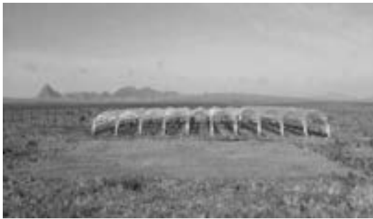
Drought experiment with a rain shelter in a Mongolian grassland during the summer of 2005
