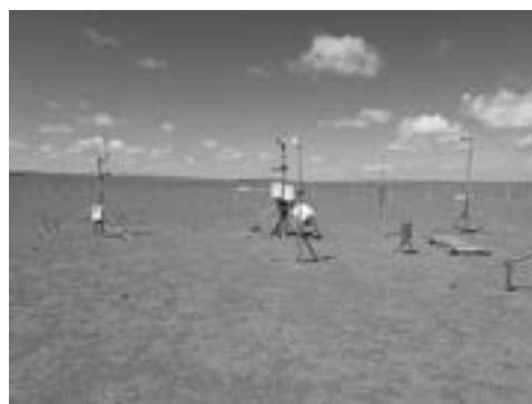
Dust emission observation system set up in Tsogt-Ovoo Mongolia located in a northern part of the Gobi Desert.
