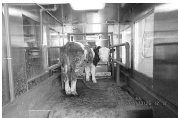
Respiratory chambers were used to measure the energy metabolism of beef cattle in China.
