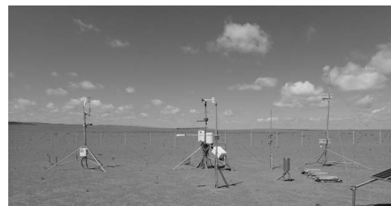
Dust emission observation system set up in Tsogt-Ovoo Mongolia located in a northern part of the Gobi Desert.
