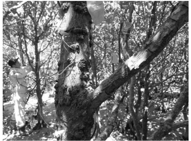
Sap flow sensor installed into mangrove trees.
