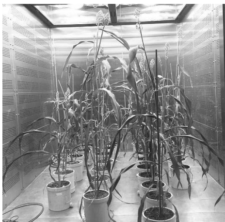
Evaluation of the Sudanese sorghum under drought inside fully controlled growth chambers.
