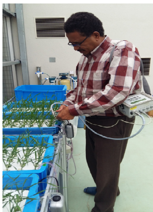
Fig1: measurement of chlorophyll fluorescence of bread wheat genotypes tested under different levels of salinity, using Mini
