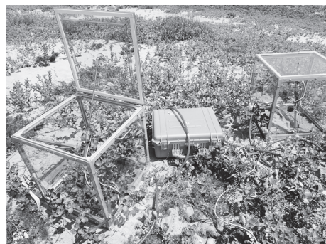
\text{CO}_2 flux measurement in a coastal dune ecosystem in Tottori
