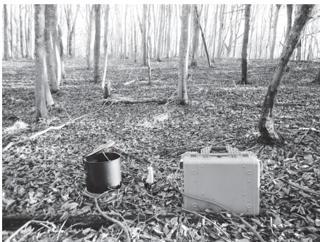
Measurement for soil \text{CH}_4 flux in a beech forest site in Hiruzen
