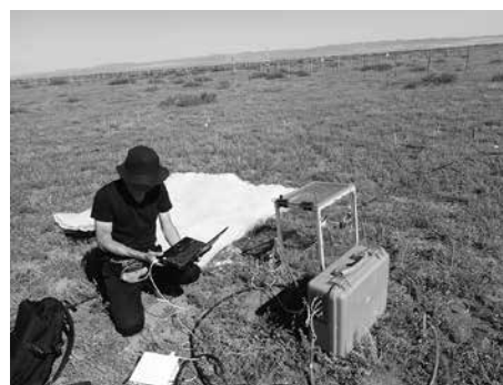
CO 2 flux measurement in a grassland ecosystem in Bayan-Unjuul
