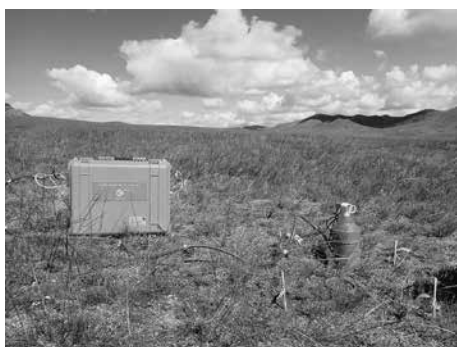
Measurement for soil respiration in a grassland ecosystem in Hustai
