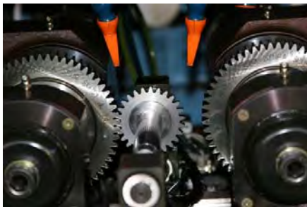
Fig.12 Configuration of plunge tool and sintered metal gear installed in rolling apparatus
