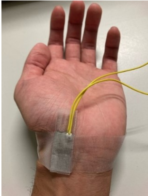
Figure 2: Piezoelectric element taped to the wrist.
