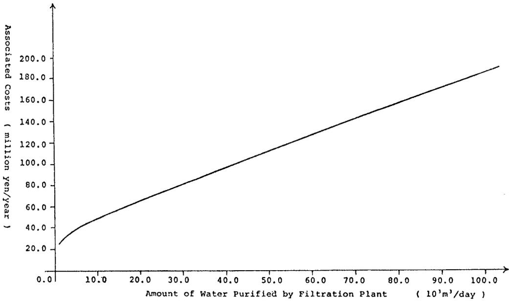
Fig. 2 Cost-scale relation for filtration plant
