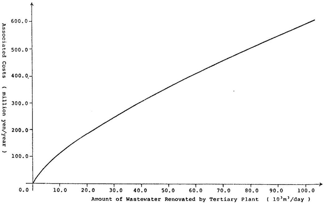
Fig. 3 Cost-scale relation for tertiary treatment plant
