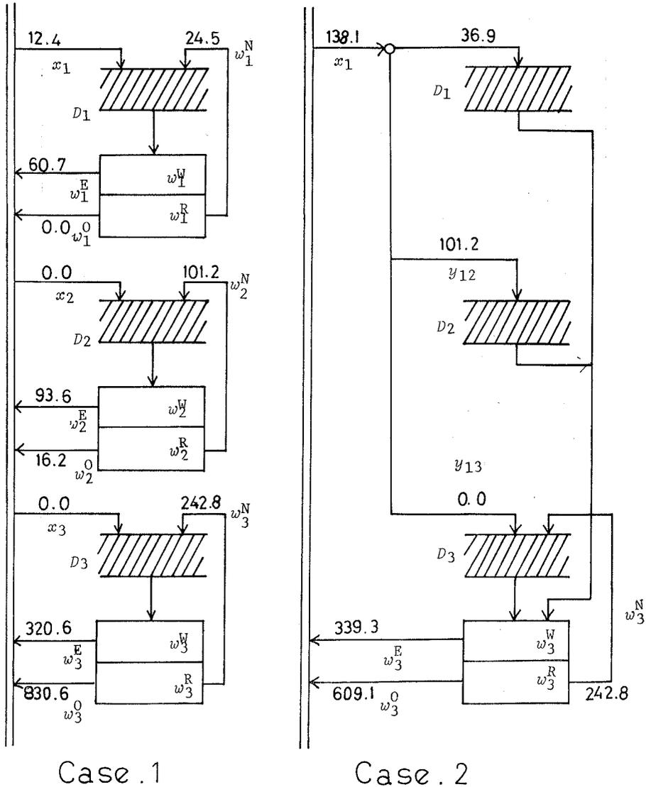
Fig. 4 Calculated water utilization patterns
