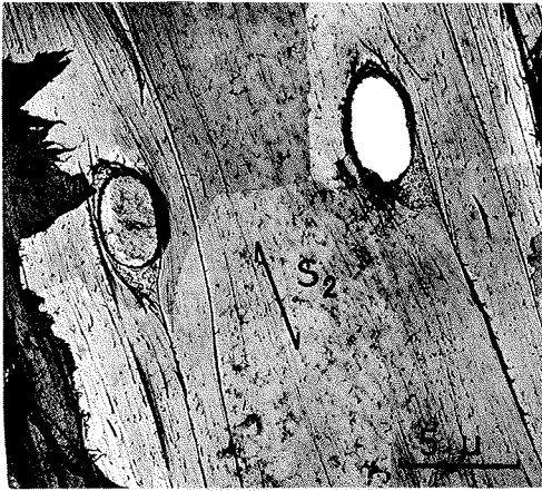
Fig. 2 Direct carbon replica of the inner surface of the cross field in a late earlywood tracheid of SUGI wood showing the microfibrillar orientation of the middle layer of the secondary wall ( S_2 ) in the vicinity of the pit aperture.
