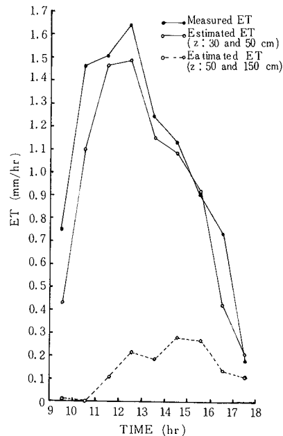
Fig. 4. Hourly distribution of measured and estimated evapotranspiration with the aerodynamic method on Aug. 29, 1971.
