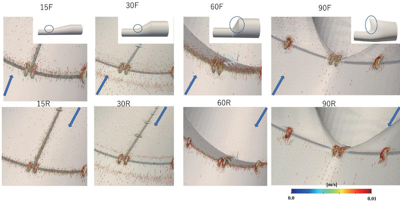
**Fig. 4.** Visualization of velocity. Vectors of  $< 0.01$  m/s are displayed. The arrows indicate the direction of flow.
