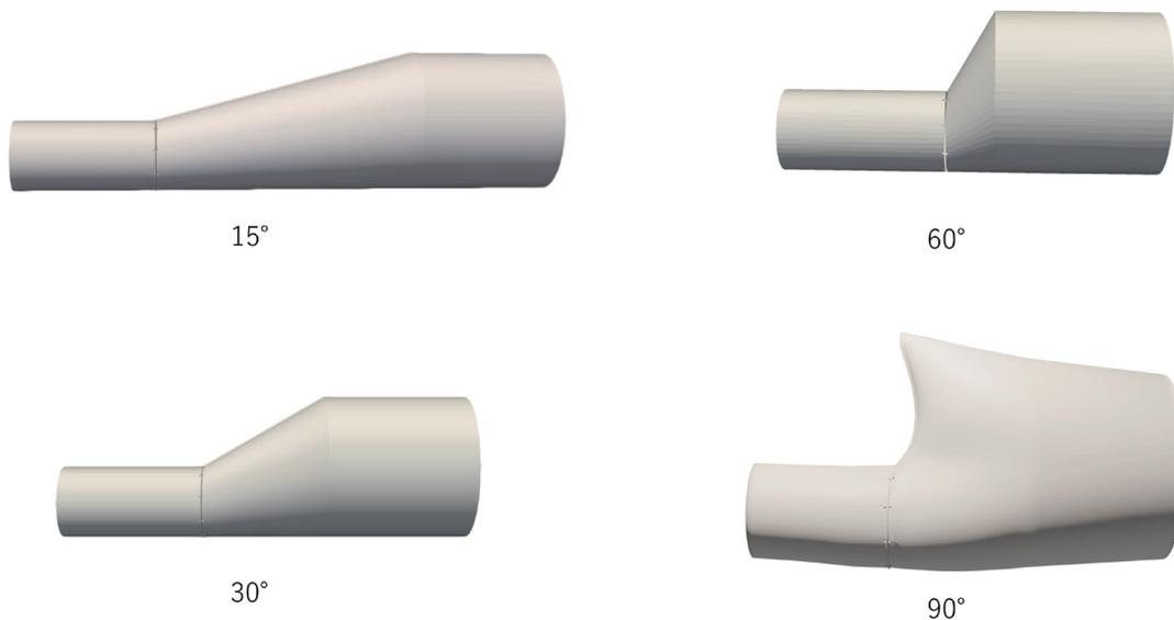
**Fig. 2.** Models with tapering at 15°, 30°, 60°, and 90°.
