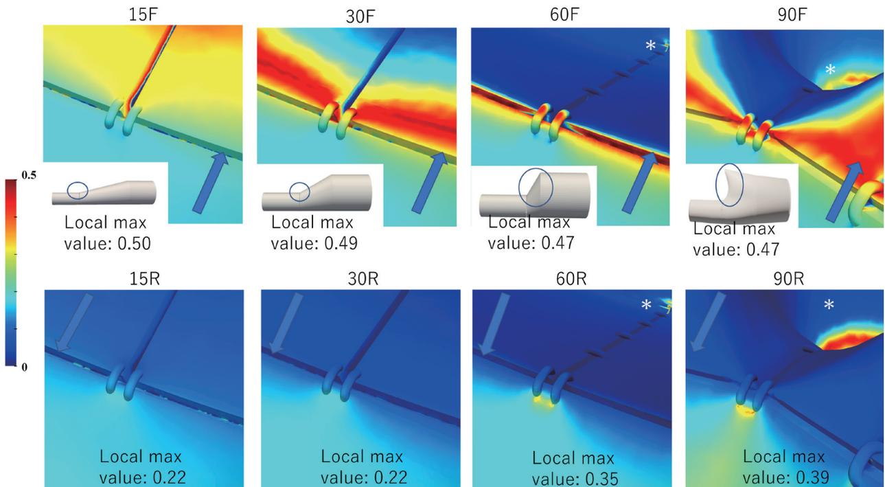
**Fig. 6.** Oscillatory shear index (OSI). The arrows show the direction of flow. For the 60F pattern, the site of the local maximum OSI value is at the peak of the suture thread of the three-point suture and along the vascular anastomosis. For the 60F, 90F, and 60R, 90R patterns, the OSI is also high at the tip of the tapered portion (\*).
