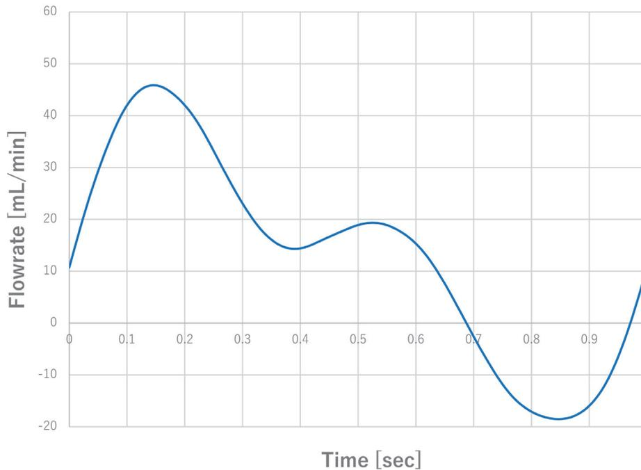
**Fig. 3.** Model venous perfusion. This is set so that the minimum value is  $-19$  mL/min at  $0.84$  s, and the maximum value is  $45$  mL/min at  $0.14$  s. The mean value is  $13$  mL/min, and 1 cycle lasts for  $1$  s.
