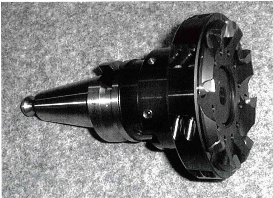
Figure 6.7 Facemill cutter for ultra high-speed cutting of cast iron
