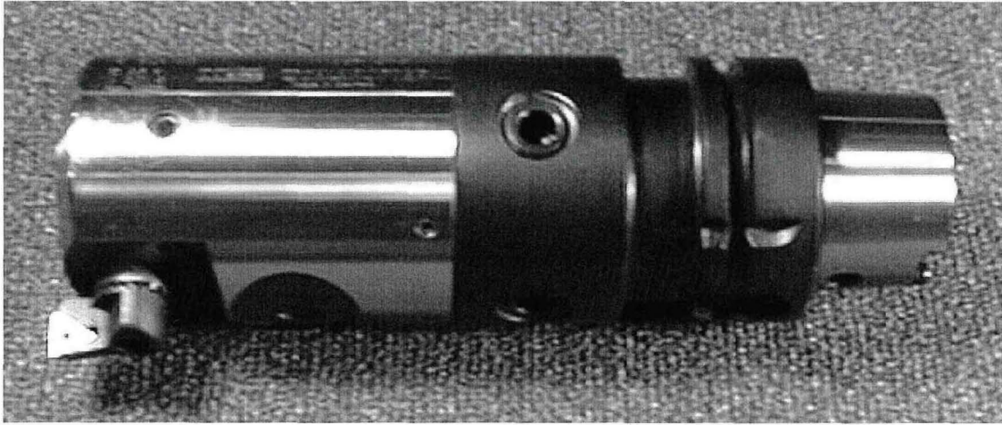
Figure 6.12 Boring bar for high-speed cutting of cast iron
