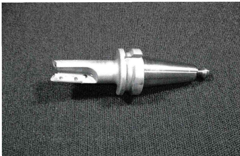
Figure 6.3 Insert type endmill for high-speed cutting of aluminum alloy
