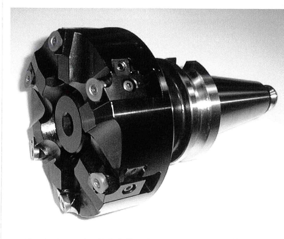
Figure 6.13 Facemill cutter for high-speed cutting of carbon steel
