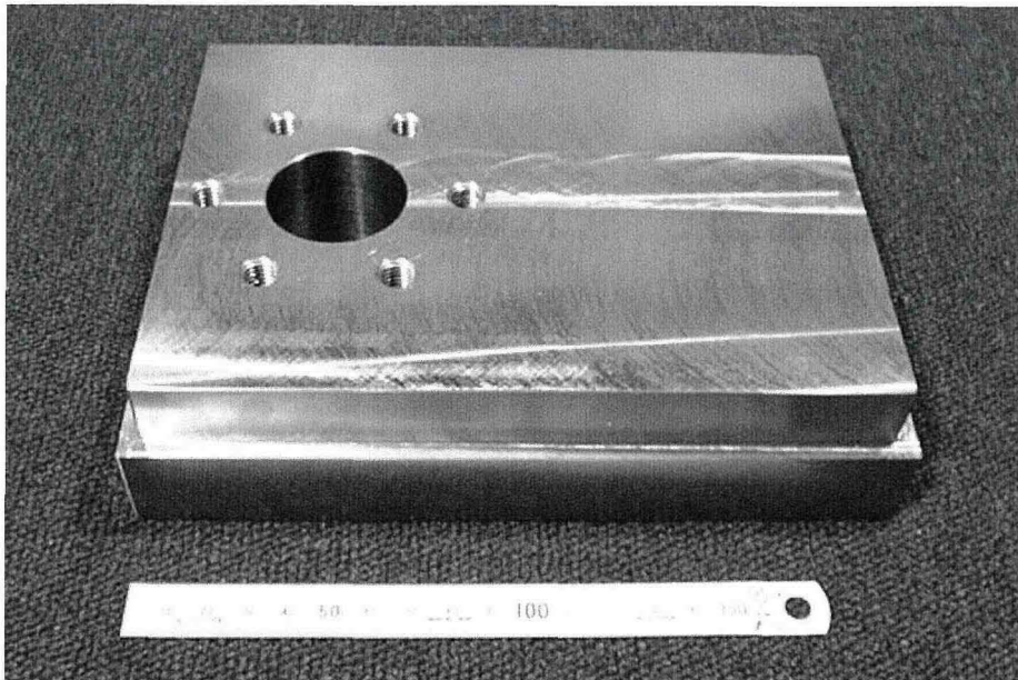
Figure 2.10 Workpiece of cycle time analysis (machine tools part) Workpiece material: S45C, 200 mm×150 mm×65 mm
