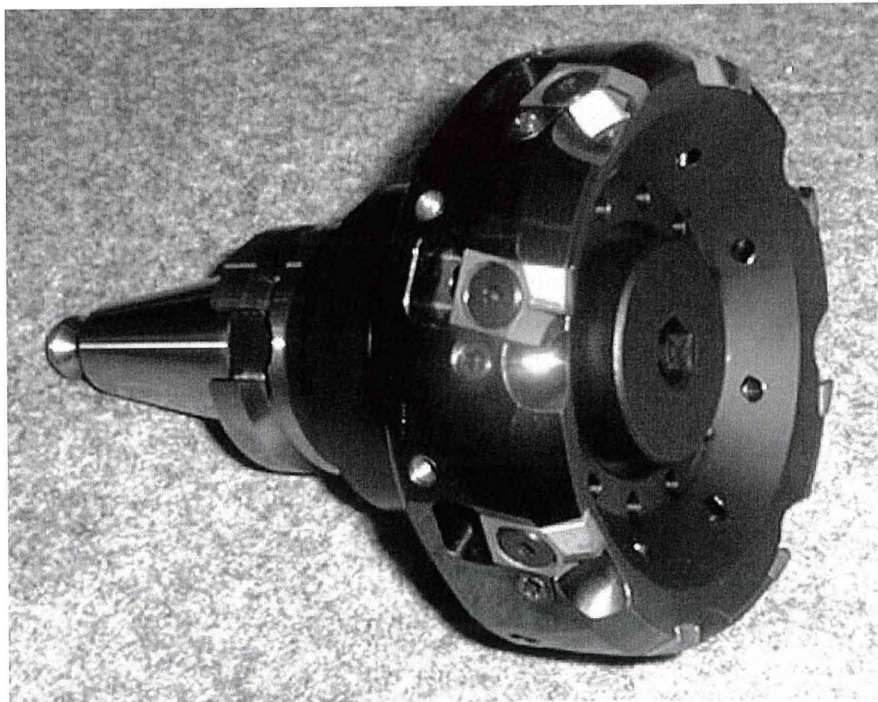
Figure 6.1 Facemill cutter for ultra high-speed cutting of aluminum alloy
