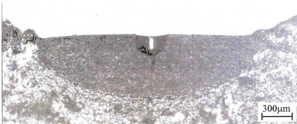
Fig. 8.7 Appearance of crack section (A2017)
