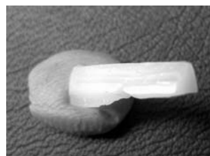
(c) Tooth (fatigue breakage)
