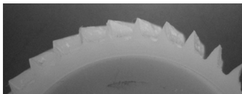
Fig.4.27 Abrasion of meshing tooth surface
