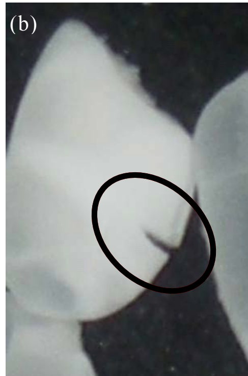
Figure 19. Reference criterion of soaking cracks. (a) not cracked, (b) cracked.
