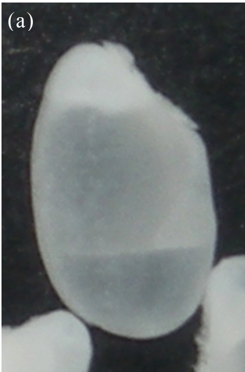
Figure 19. Reference criterion of soaking cracks. (a) not cracked, (b) cracked.
