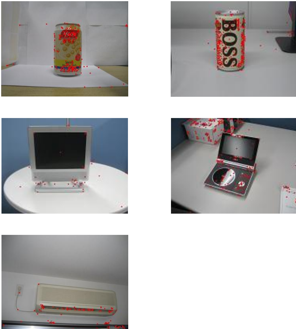
Figure 2.3.2 SIFT feature detector results for (a) a soymilk can, (b) coffee can and home appliance,(c) TV set, (d) DVD player, and (e) an air conditioner with simple shape producing a small number of SIFT feature counts compared to the coffee can.
