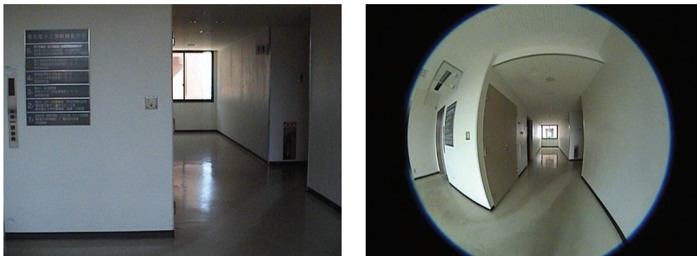
Fig 3.1 Different fields of view of images captured by a conventional camera and a fisheye camera.
