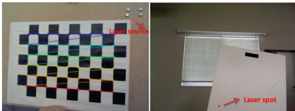
Figure 5.4: Example images. Left is the laser source on the pattern captured by Camera 1 inside the vehicle. Right is the laser spot captured by Camera 2 outside the vehicle (in an ordinary scene).
