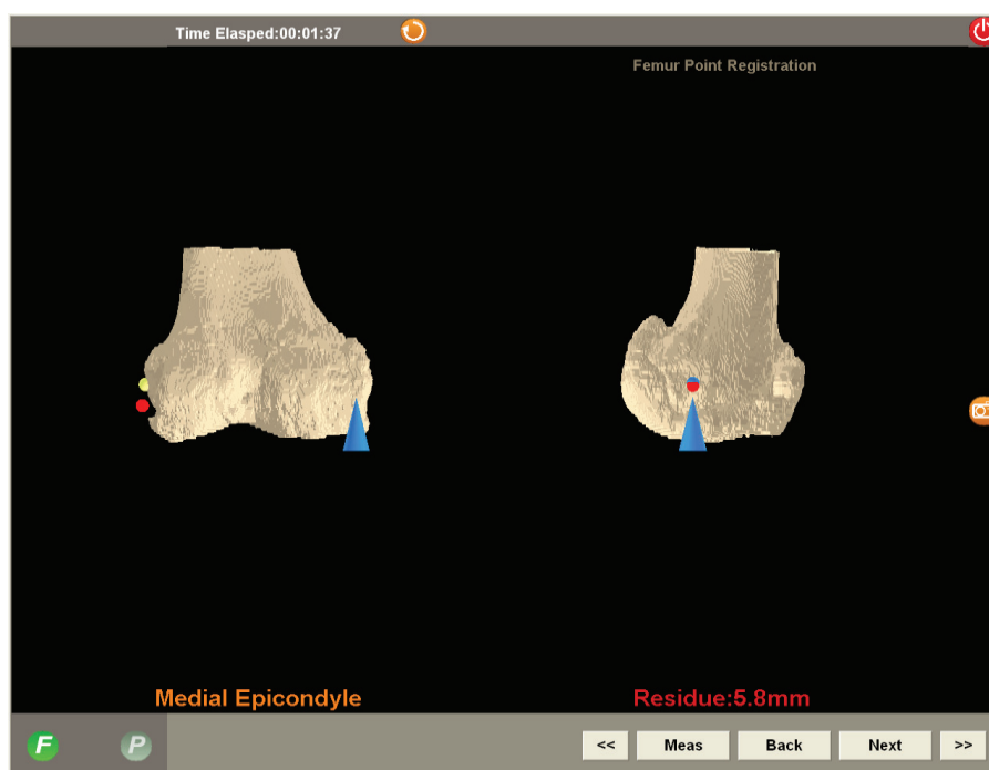
Fig 4-14 Femur point registration. The yellow point shows the preplanning landmark, the red point is the measured landmark, blue point and arrow are the current measured point.
