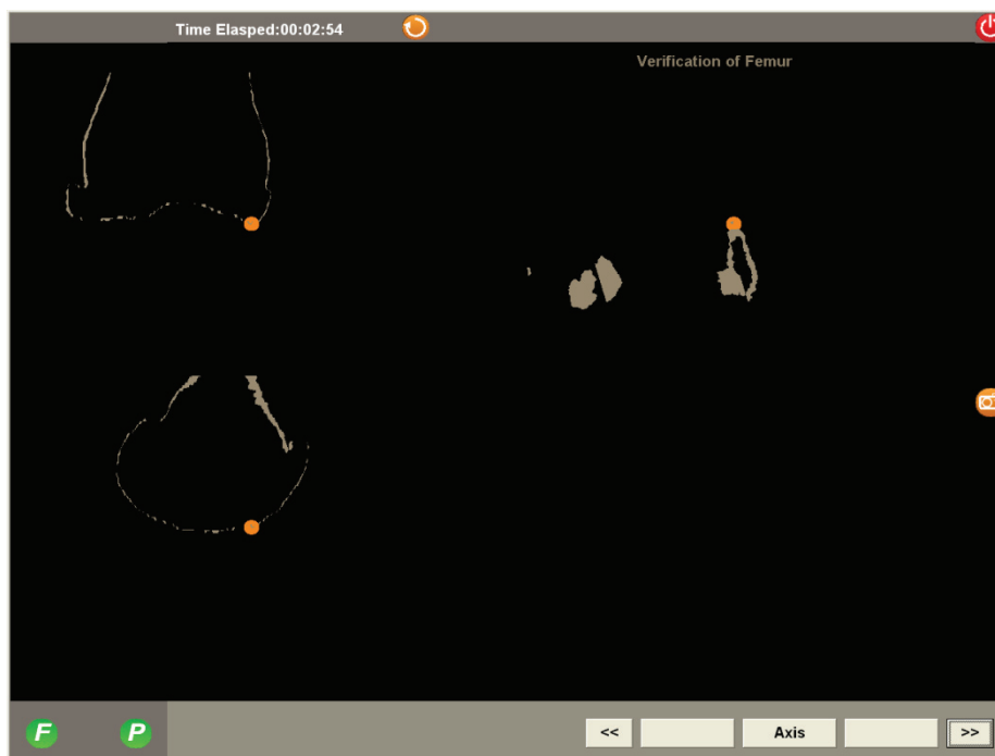
Fig 4-16 Verification of femur registration. The white lines show the coronal, sagittal and transverse contour of virtual femur, the orange points indicate the position of probe tip which translated from real to virtual space.
