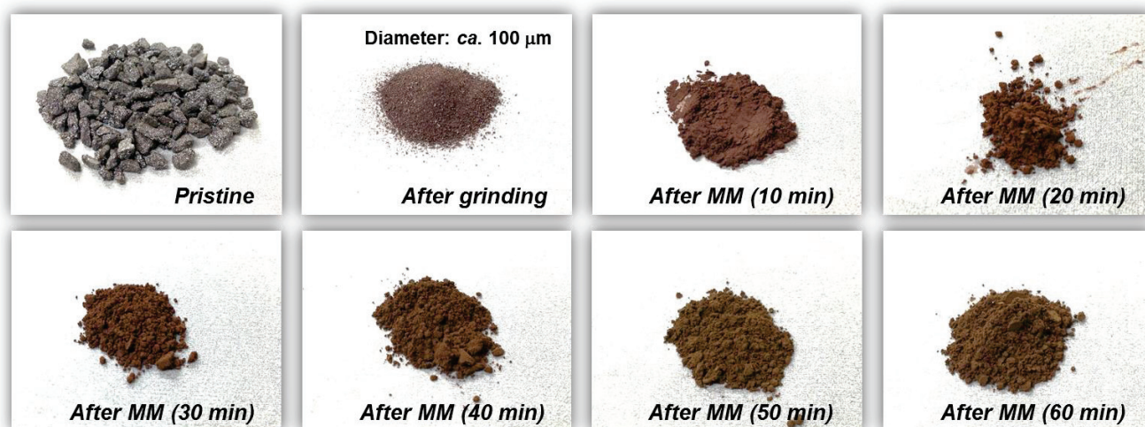
Figure 6-1. Photographs of various silicon monoxide (SiO) powders. A granular SiO with a diameter of 2–3 mm (Wako Pure Chemical Industries, Ltd.) was pulverized by using a high-energy planetary ball mill (Classic Line P-6, FRITSCH) at 380 rpm to prepare an active material powder. The weight ratio of the balls to the powder was set to be 65:1, and the mechanical milling (MM) times were 10 min, 20 min, 30 min, 40 min, 50 min, and 60 min, respectively.
