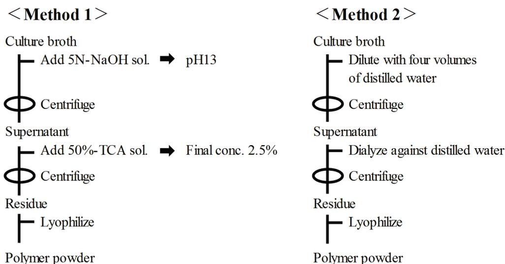
**Figure 12 Purification methods of BL58 polymer**
