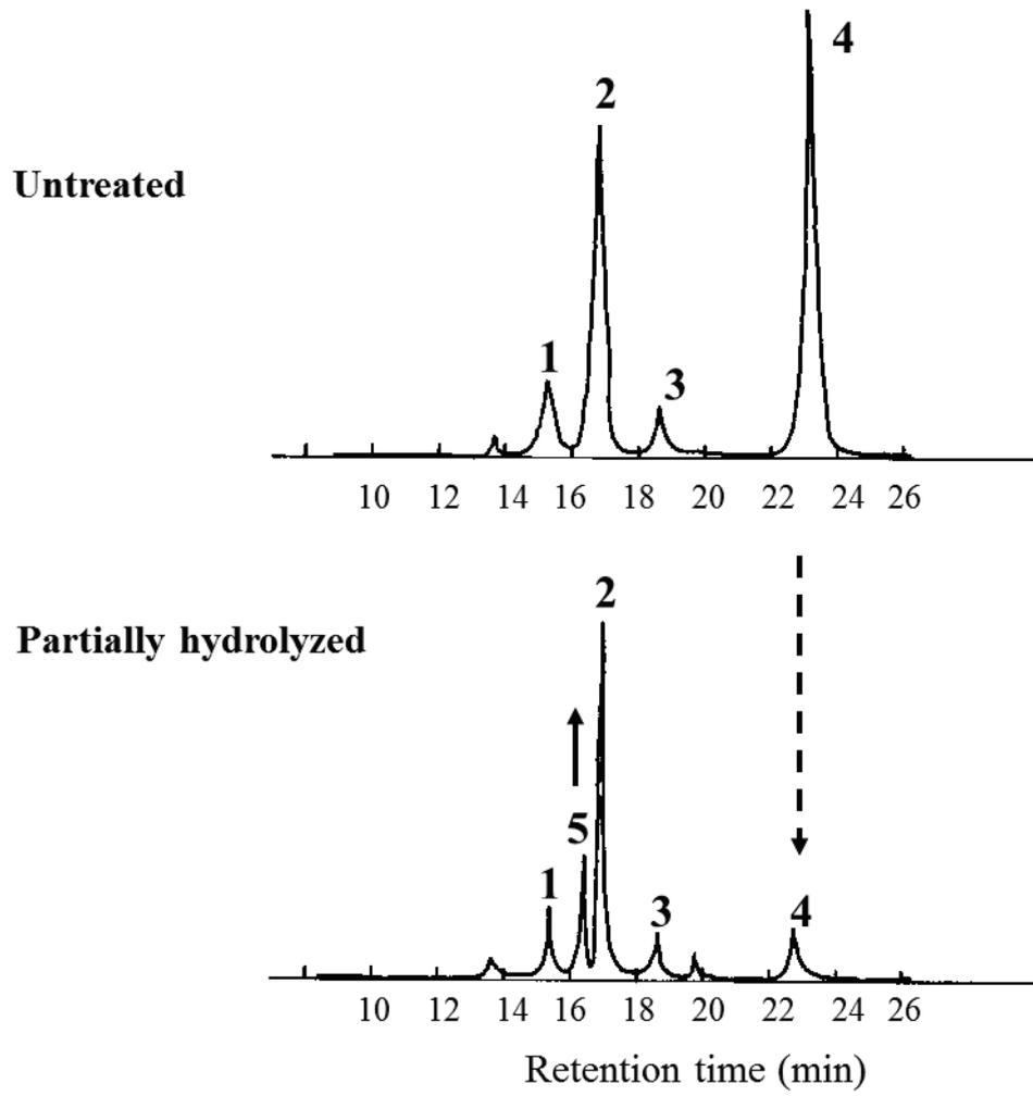
Figure 19 GC-MS analysis of partially hydrolyzed BL58 polymer
