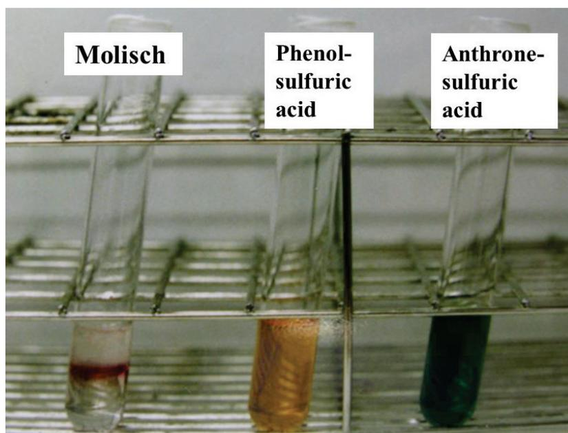
**Figure 5 Color reaction tests for sugar**
