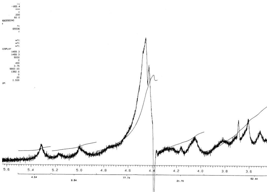
**Figure 16** 600-MHz  $^1\text{H}$ -NMR spectrum of native BL58 polymer at 60°C
