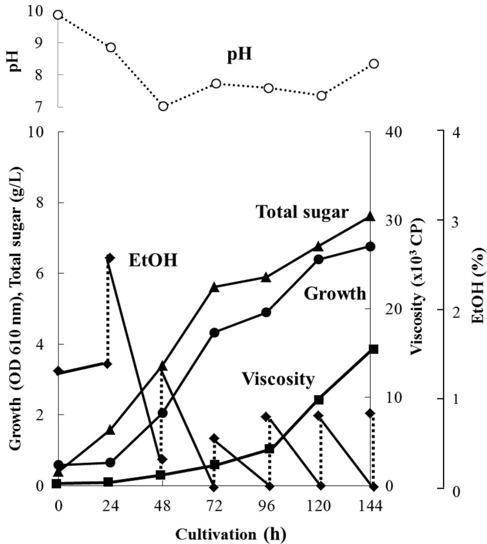
Closed rhombus indicate ethanol, close squares viscosity, closed triangles total sugar, closed circles growth (OD 610 nm) and open circles culture pH
