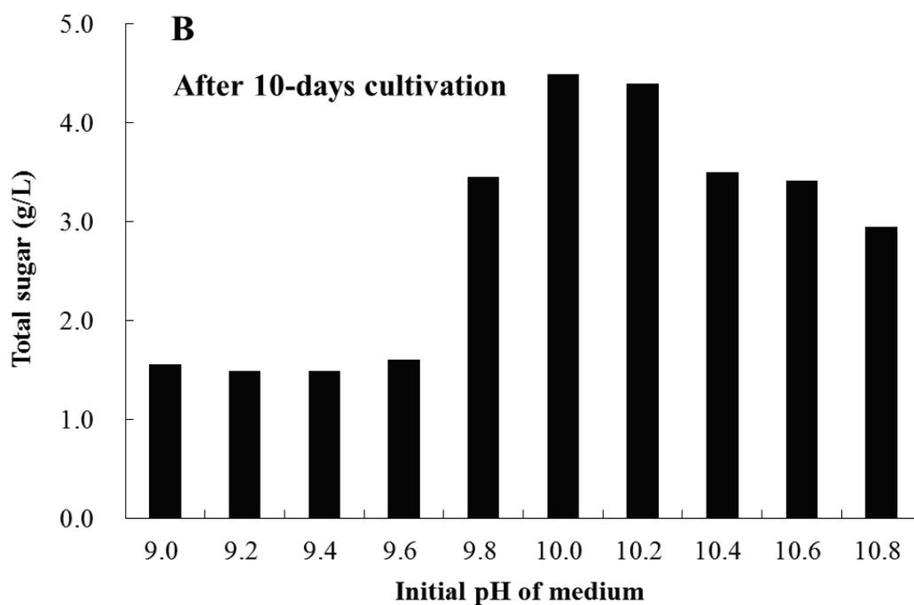
**Figure 6 Effect of initial pH on growth and BL 58 polymer production**
