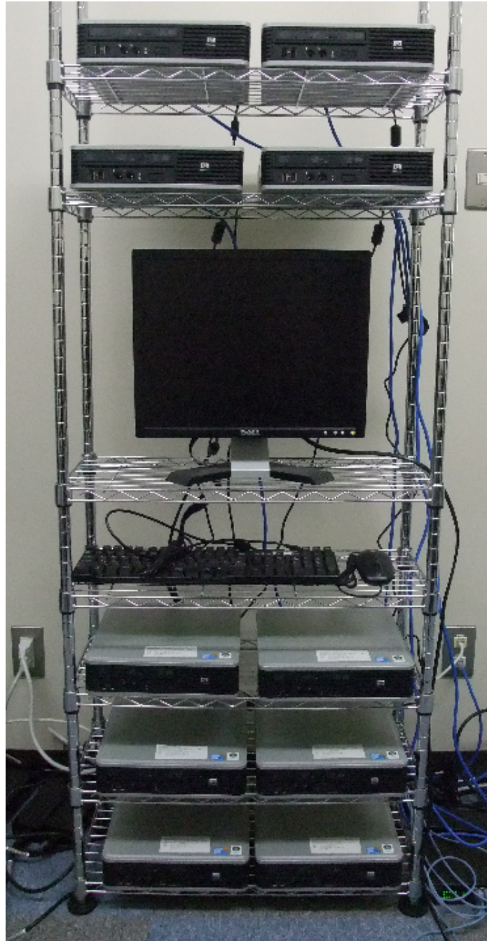
Figure 2.4: Installation of used-computers using an aluminum rack.
