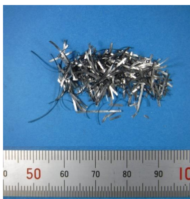
Figure 2-1. Photograph of silicide/Si composite ribbon prepared by rapid quenching method.
