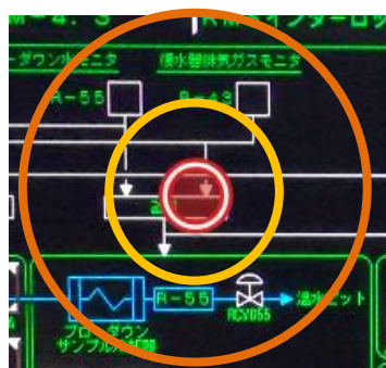
Red circle: Textual/numerical character detection area Yellow circle: Symbols detection area Orange circle: Color detection area
