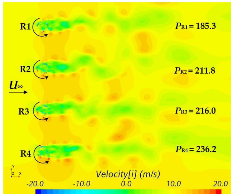
Fig. 2 Unsteady flow field ( $x$ -component) around the four-rotor parallel layout simulated by CFD analysis using the DFBI model ( $U_\infty = 10$  m/s, inter-rotor space ( $gap$ ) =  $3.0D$ )
