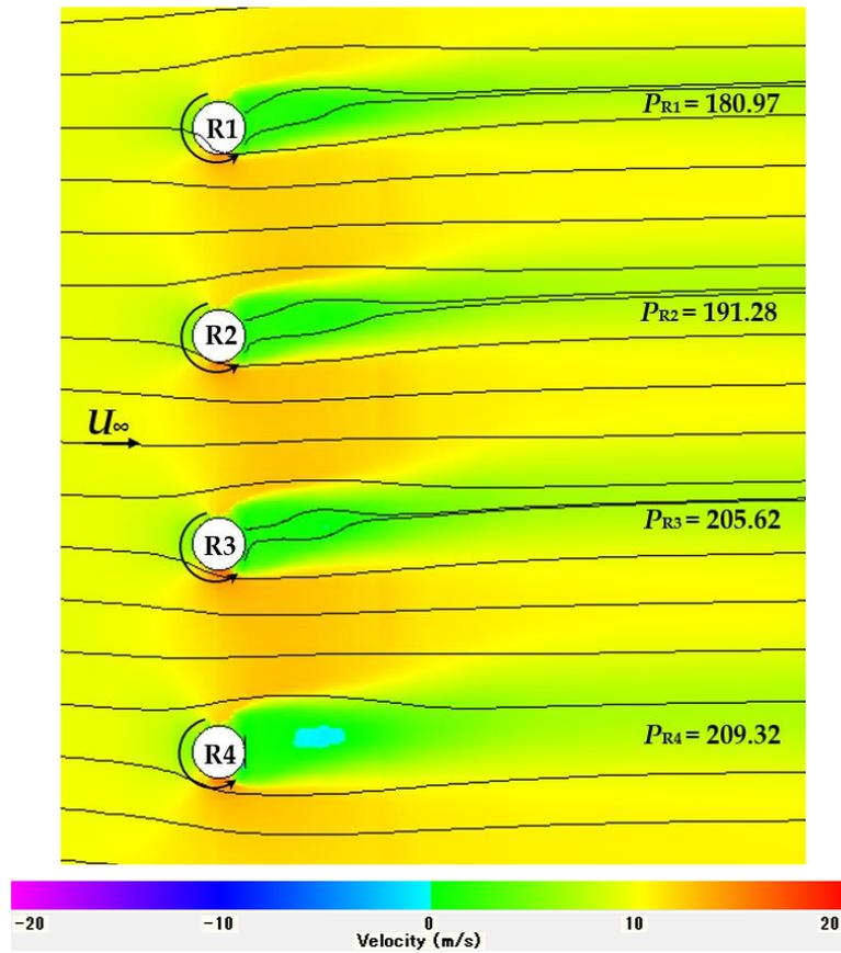
Fig.1 Prediction by the proposed method of the averaged distributions of  $x$ -direction velocity components around four-rotor parallel layout ( $U_\infty = 10$  m/s, inter-rotor space ( $gap$ ) =  $3.0D$ )
