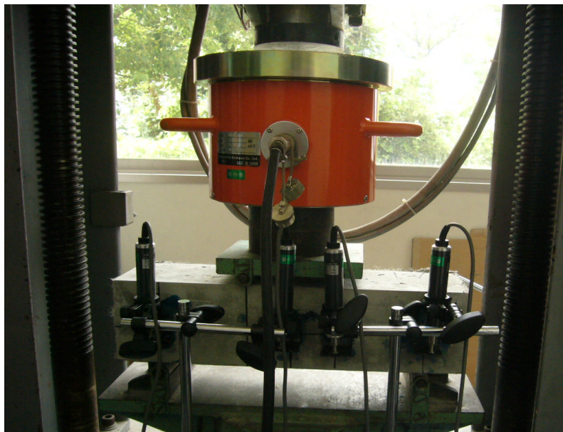
Fig.5-9 荷重—変位試験 Load-deflection test configuration
