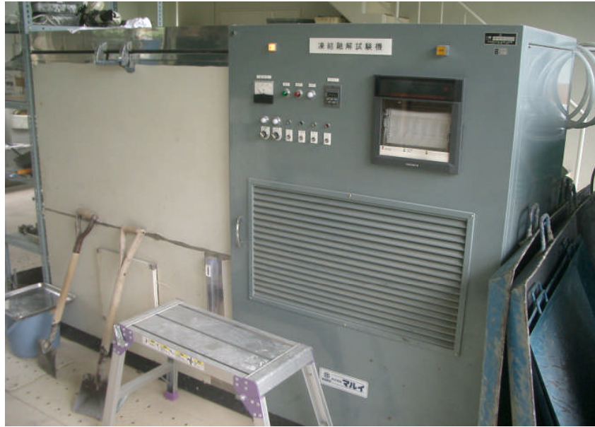
Fig.4-3 凍結融解試験機 (B 法) Freezing and thawing test (for A method)
