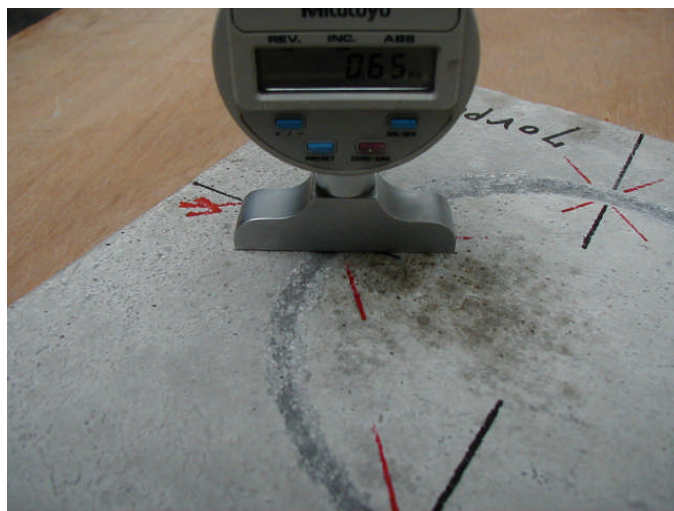
Fig.3-8 摩耗深さの測定 Measurement of the abrasion depth
