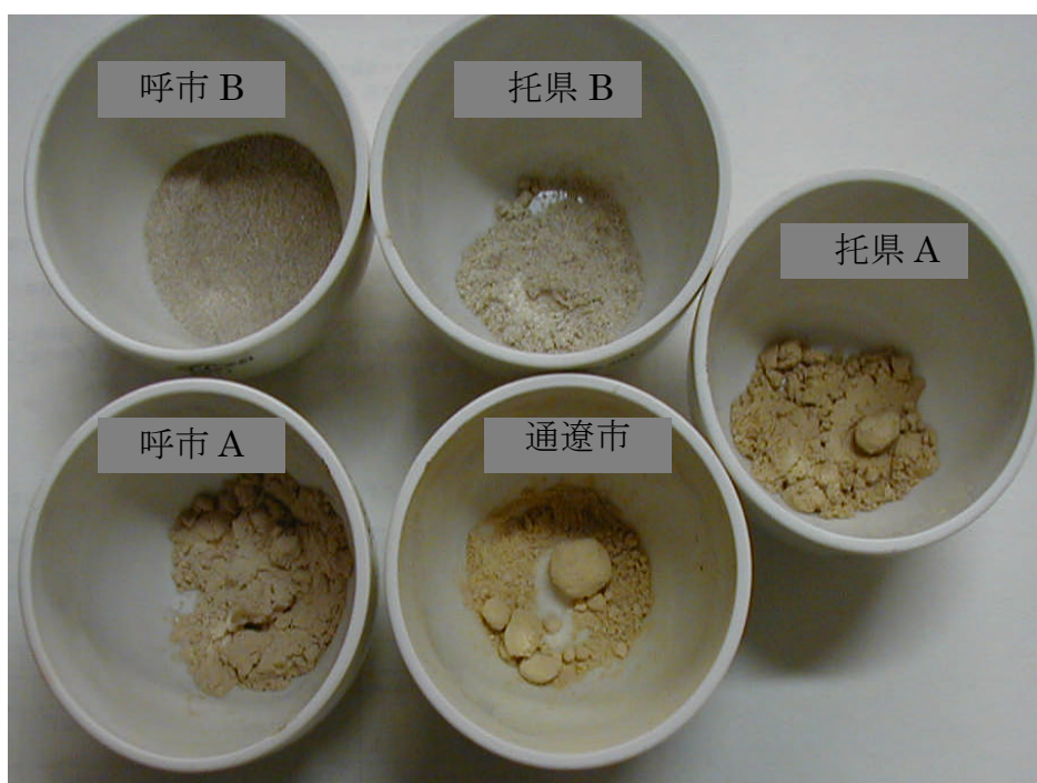
Fig.2-5 電気炉で強熱後のフライアッシュ After the ignition of the electric furnace with fly ash
