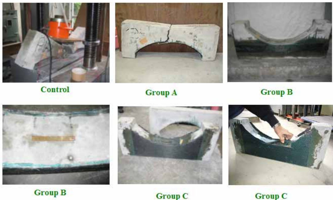
Photo 5.3: Modes of failure for the examined arch specimens
