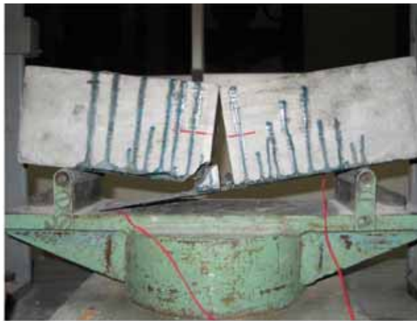
Photo 3.5: Interfacial debonding in case of concrete substrate
