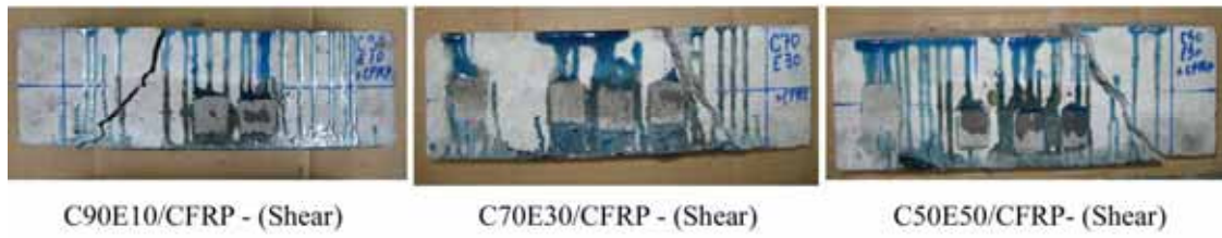
Photo 3.9: Modes of failure for small specimens
