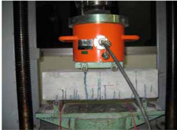
Photo 3.4: Typical indirect tension test configuration
