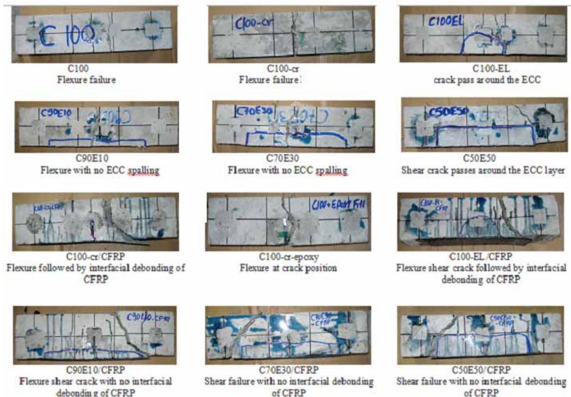
Photo 4.2: Typical Modes of failure for the examined specimens
