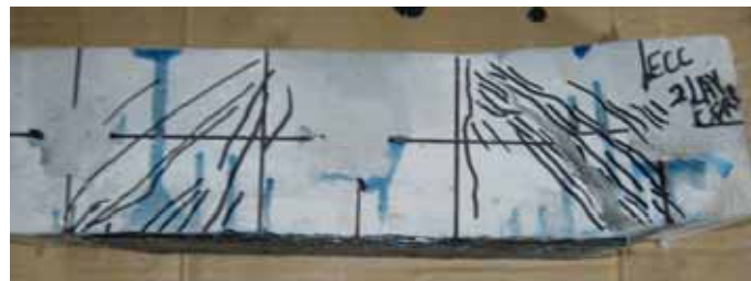
Photo 3.7: Shear failure mode for ECC beam strengthened with CFRP
