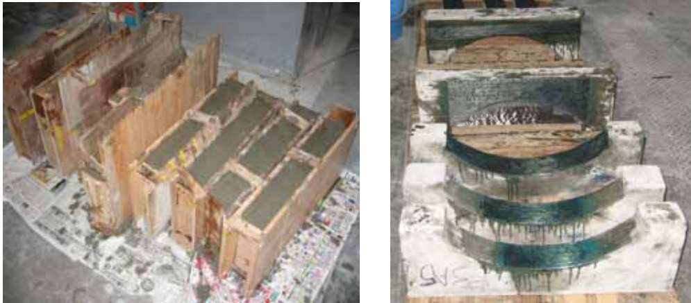
Photo 5.1a): Moulds after casting, and b): after pasting CFRP sheets
