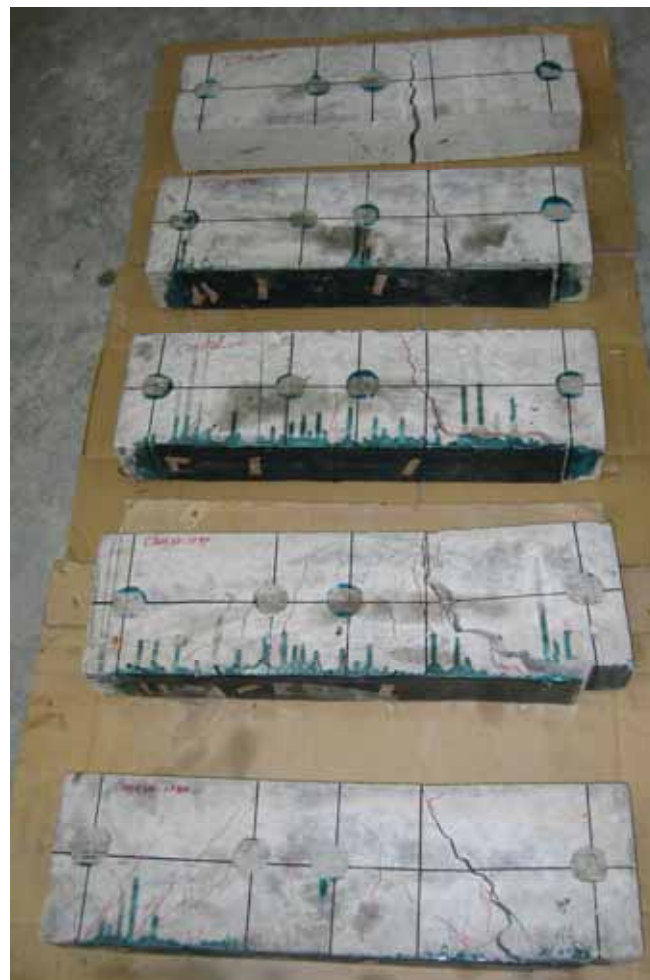
Photo 3.10: Modes of failure for big specimens
