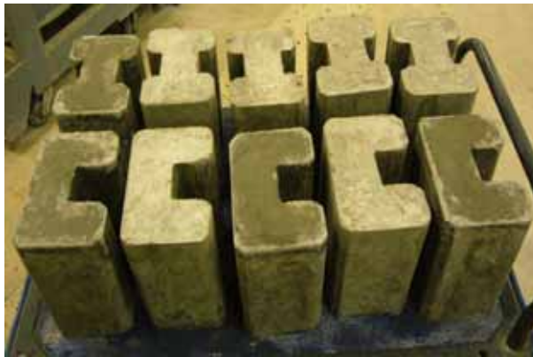
Photo 6.2: Concrete prisms after casting
