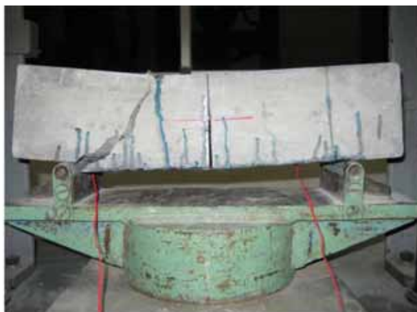
Photo 3.6: Shear failure in case of ECC substrate
