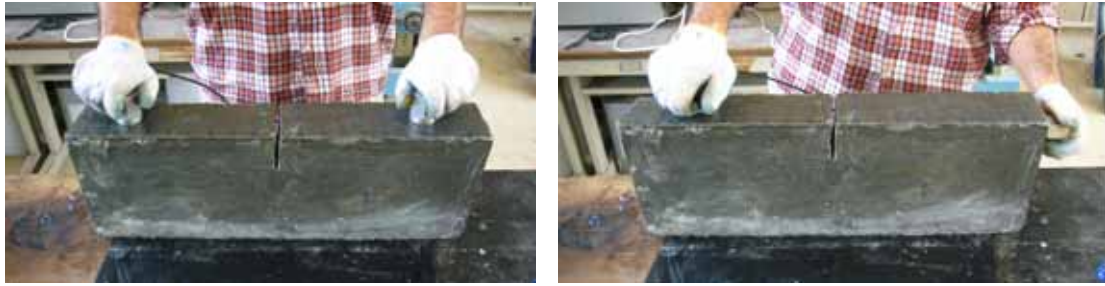
Photo 2.2 a): Indirect transmission and, b): Semi-direct transmission for UPV test
