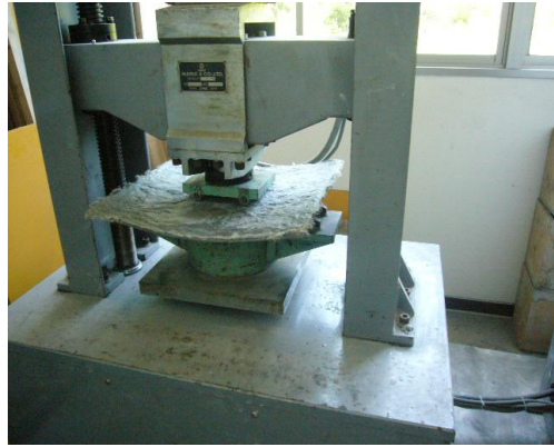
Fig.3.1.1. Generation of cracks using a bending machine
