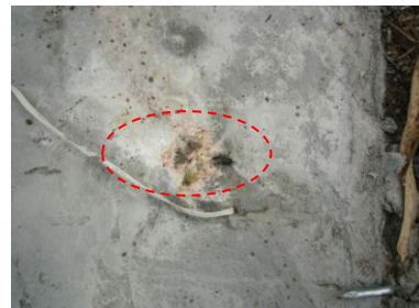
Fig.3.2.9. Disaggregated sand and cement on previously unstiffened patch on mortar 21 days after casting
