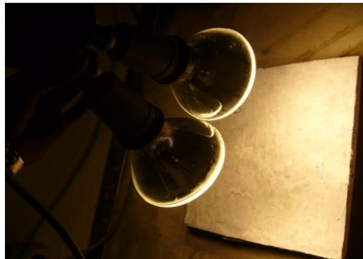
Fig.3.1.2. Illumination of an ECC plate by 2 tungsten bulbs, each with wattage of 150W
