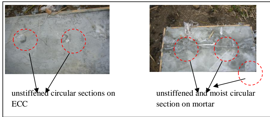
Fig.3.2.7. ECC and ordinary mortar plates 24 hours after casting
