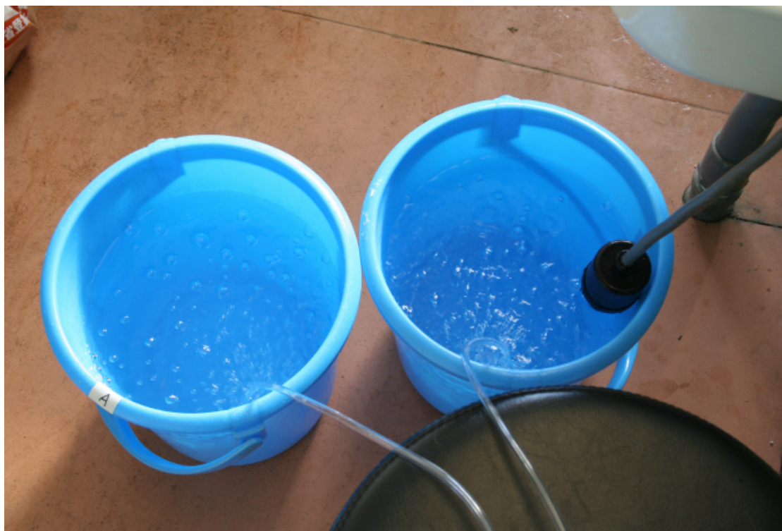
Fig. 2. Electro-degradation (ED) of nutrient solution with benzoic acid with constant aeration in a without plant experiment.
