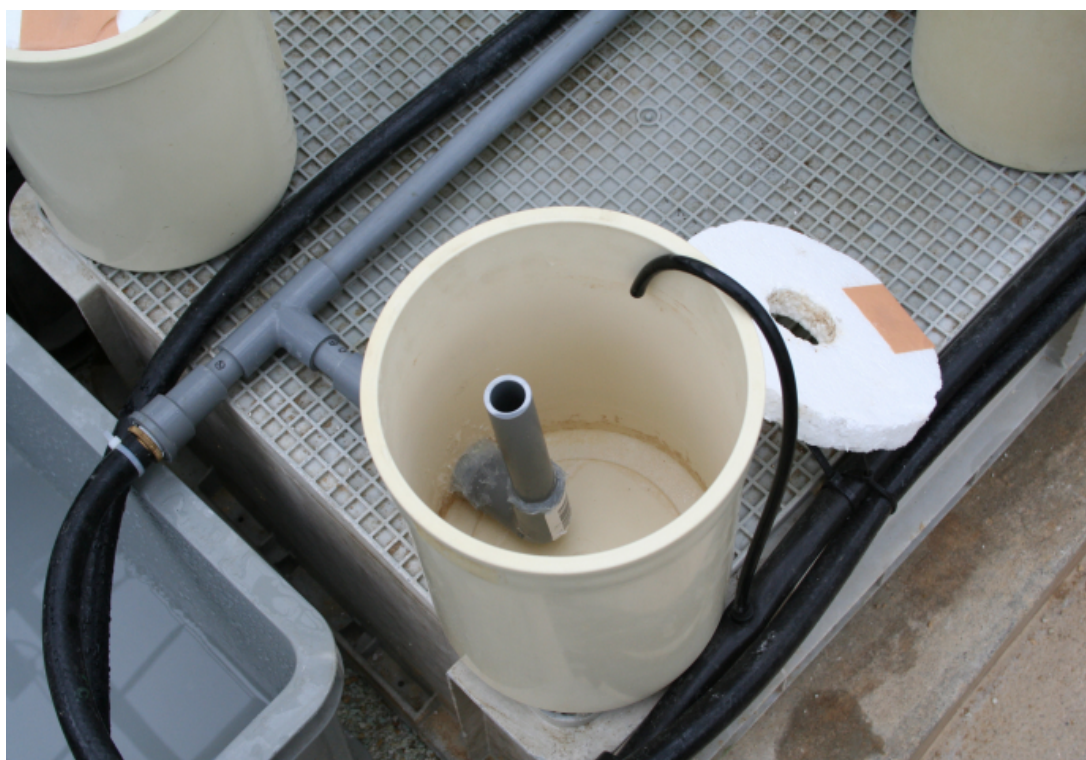
Fig. 3. Wagner's pot with capacity of 3 liters nutrient solution used for strawberry hydroponics in the greenhouse.
