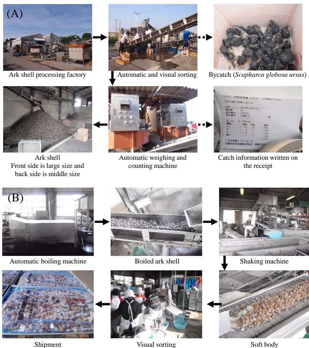
Figure 1-6. Ark shell processing factory in North Ariake Sea, Saga Prefecture. Process of weighing and counting (A); process of making stripped ark shell flesh (B).
