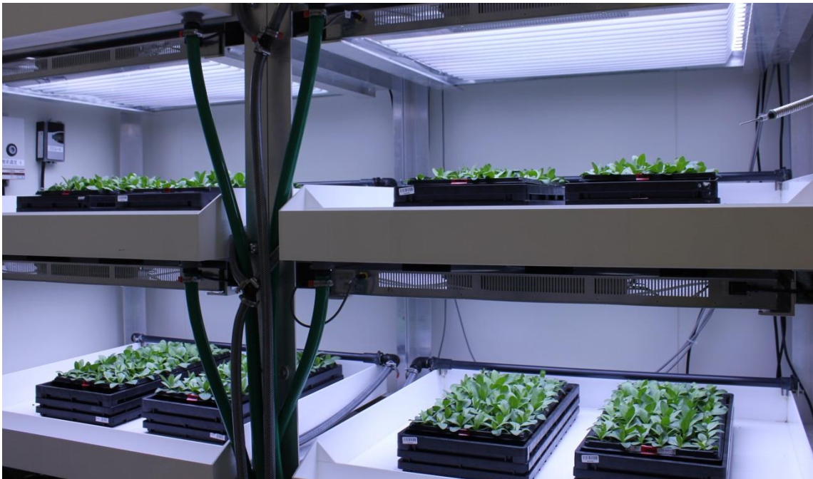
Fig. 3. Lisianthus seedlings grown in the horticultural soil under Hybrid Electrode Fluorescent Light (HEFL) inside the growth chamber.
