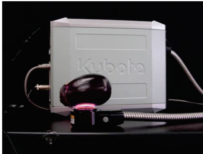
Fig. 2-5. The measurement of the NIR spectrum of a Mizu-nasu eggplant fruit using the K-BA100R spectrometer.
