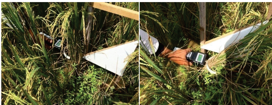
Figure 5.3. Lodging resistance measurement
