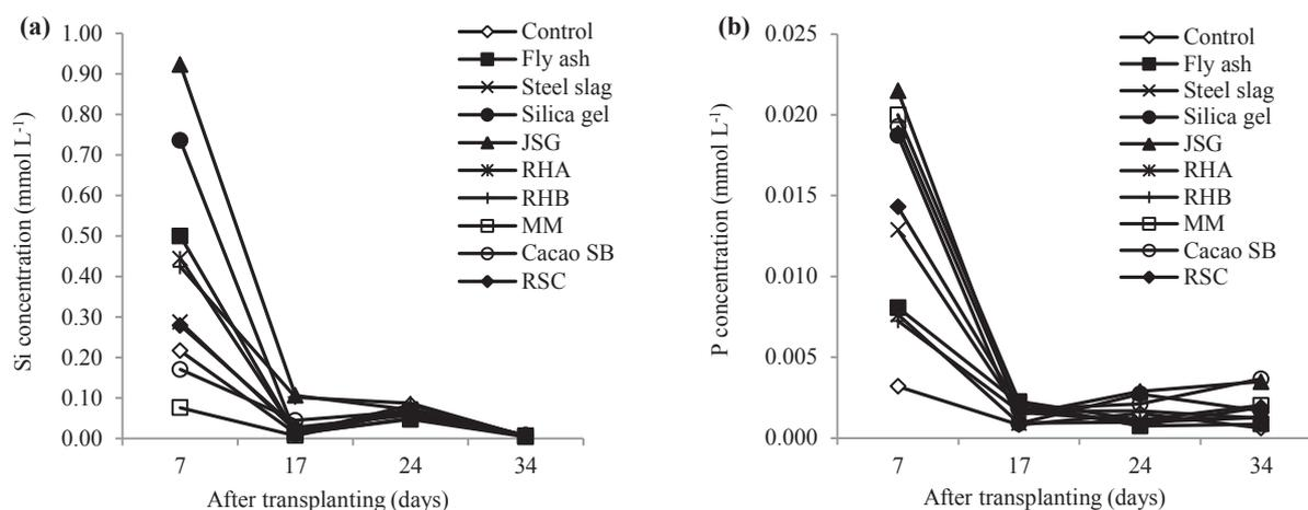
Figure 9. Release pattern of Si (a) and phosphorus (b) in soil solution during 34 days of experimental time
