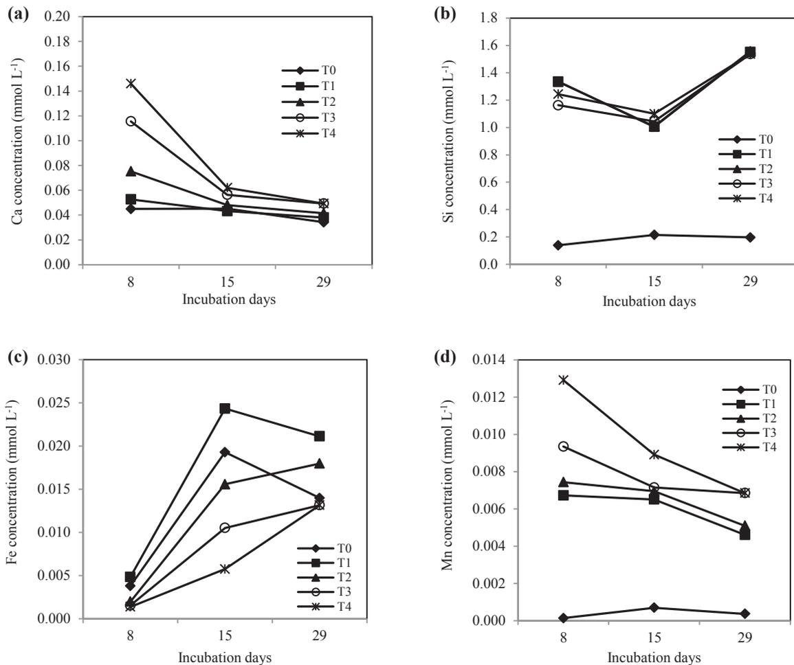
Figure 2. Release pattern of calcium (a), silicon (b), iron (c), and manganese (d) during 29 days of experimental time
