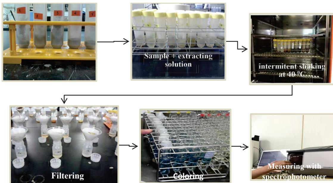
Figure 4. Acetate buffer extractable-Si
