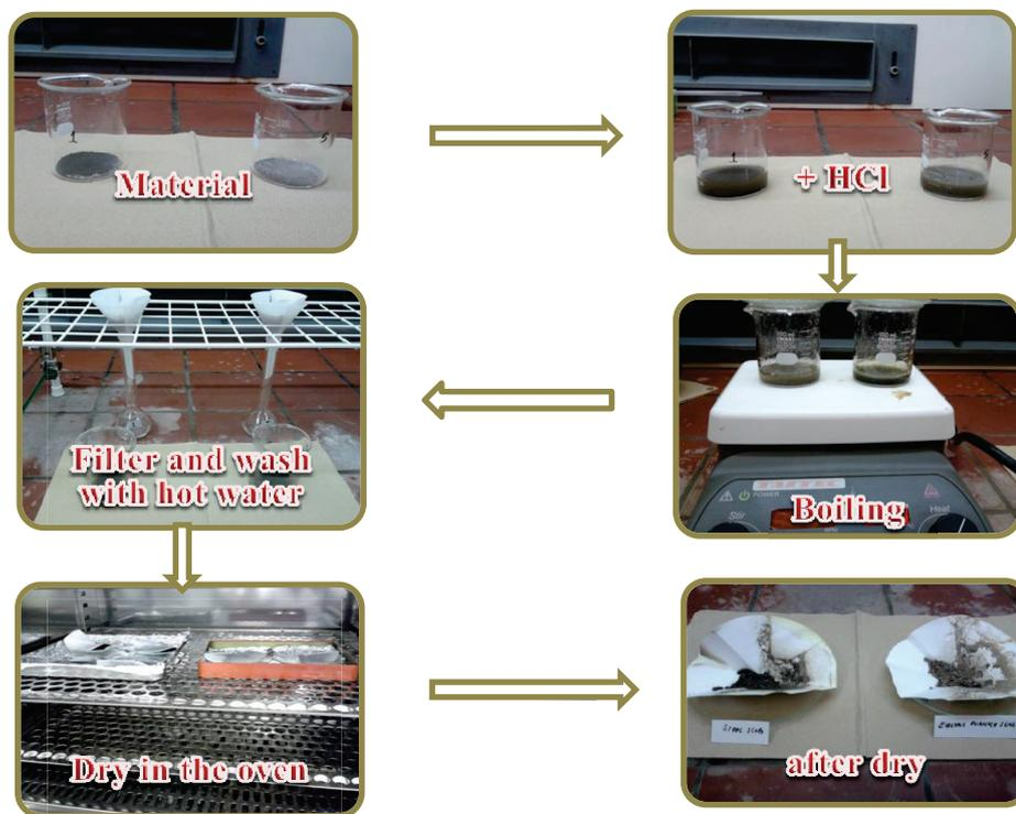
Figure 1. The flow diagram of technique 1
