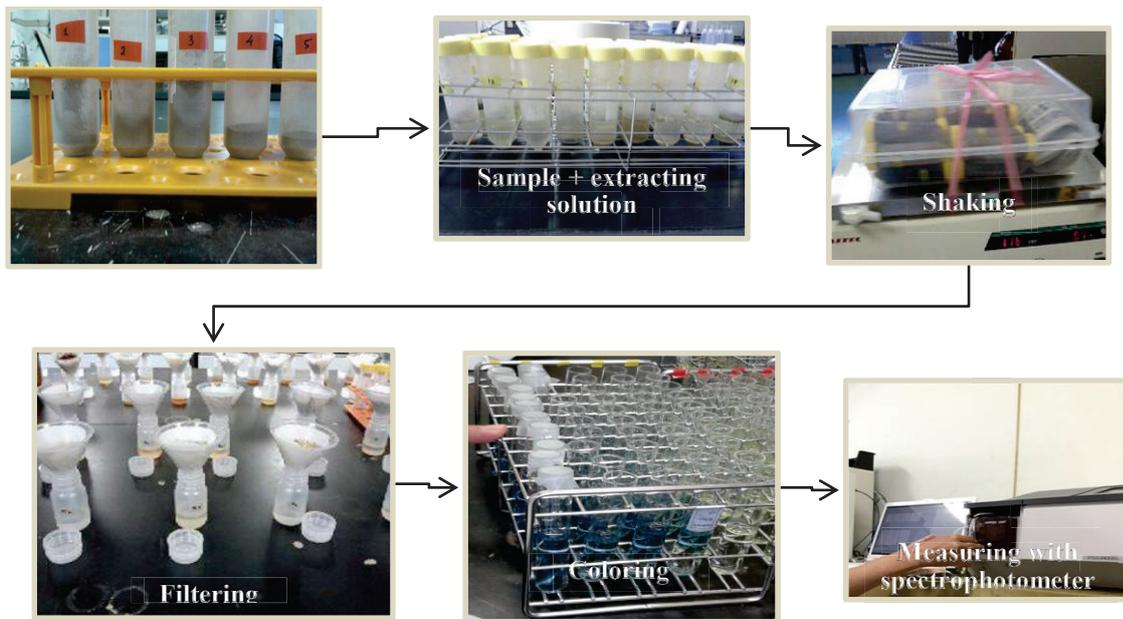
Figure 3.  $\text{Na}_2\text{CO}_3/\text{NH}_4\text{NO}_3$ , sodium phosphate, HCl, citric acid, and  $\text{CaCl}_2$  extractable-Si
