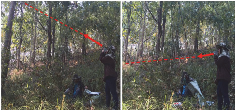
Measurement of tree height using Haga altimeter and clinometer
