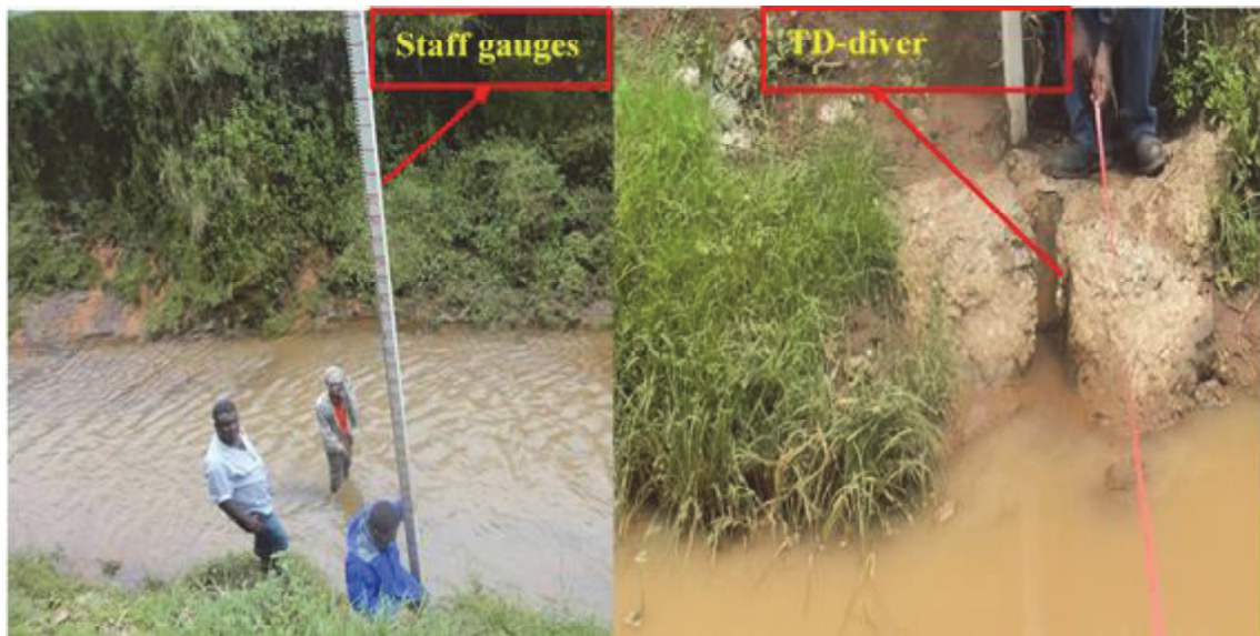
Figure 4- 2 Typical monitoring station with staff gauges (vertical poles) and a TD-diver at the deepest point of the river cross-section.
