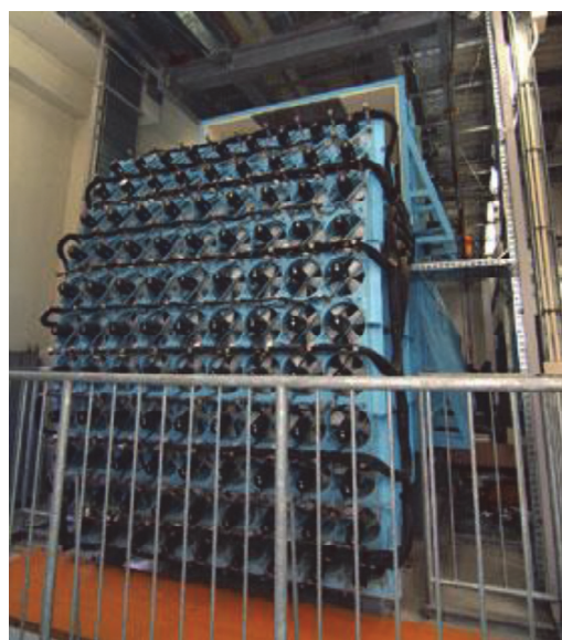
Fig 2.2 Multi-fan device in Miyazaki University
