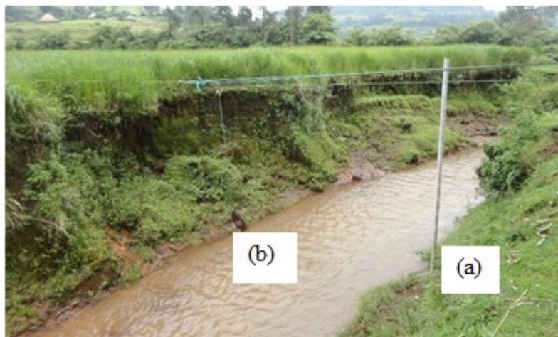
Figure 2.2 A river gauge station at the outlet of the Akusity watershed equipped with different measuring materials: (a) a staff gauge with a TD-Diver pressure transducer at the bottom, and (b) a depth-integrated suspended sediment sampler suspended from a cable stretched across the stream.
