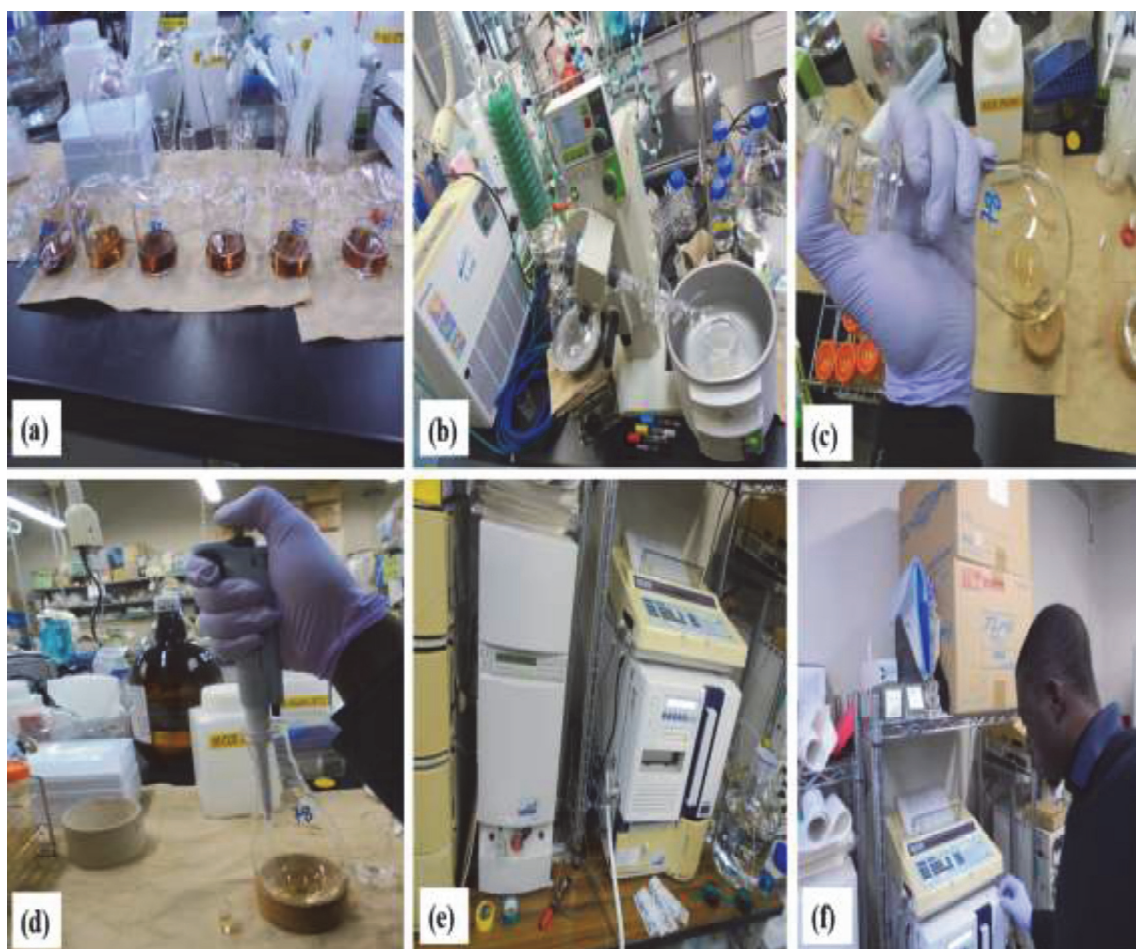
Figure 14. (a) Phenolic compound extraction with 2 M NaOH, (b) evaporation to dryness on rotary evaporator, (c) and (d) dissolving evaporated sample in 80% CH 3 OH, (e) and (f), HPLC analysis of phenolic compounds.
