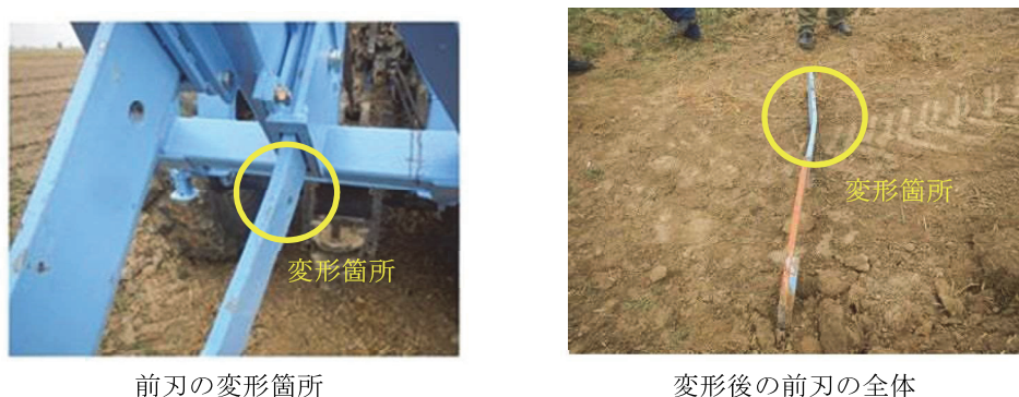
Fig. 5-18 切断刃の変形 Deformation of the cutting blade
