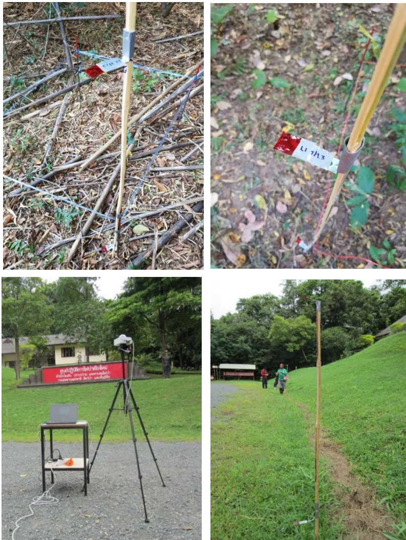
Figure 4.5 Light intensity measurement by opto leaf film and pyranometer in study area and open area.
