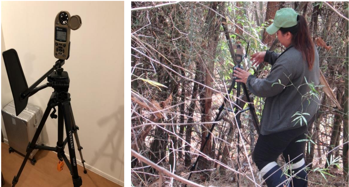
Figure 5.3 Measurement environment weather data during fire experiment by portable weather recorder (Kestrel 5500 Meter).
