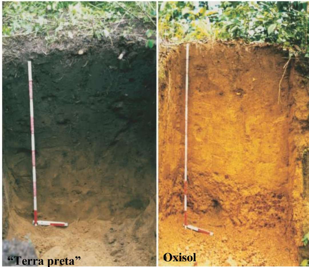
Figure 4. Typical profiles of the “terra preta” and oxisol (From Glaser et al., 2001).
